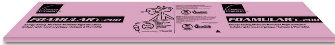
FOAMULAR® C-200's compressive resistance of 20 psi is an economical alternative to a 30 psi product for all building wall applications, including below grade exterior. FOAMULAR® C-200 maintains its R-value even when exposed to moisture typically present in the walls of buildings. For these reasons architects, engineers, contractors and owners have been specifying and applying FOAMULAR® C-200 since 1986.
